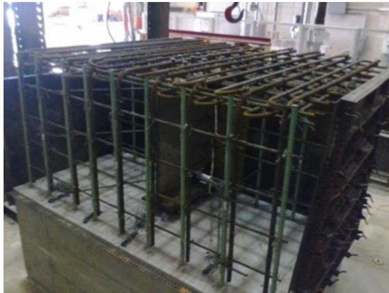
Figure 2.44 Cast-in place integral diaphragm. (Hosteng, Phares, & Redd, 2016)
