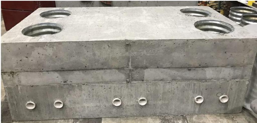
Figure 4.44 Pile coupler pile cap completed.
