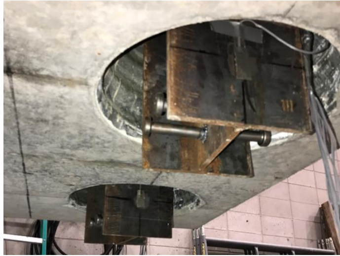
Figure 4.56 Steel sections suspended within integral diaphragm CMPs.
