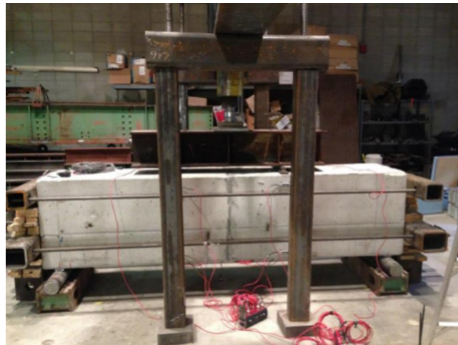
Figure 2.40 Specimen setup for static four-point bending test with applied axial load. (Hosteng, Phares, Abu-Hawash, Bierwagen, & Nelson, 2015)
