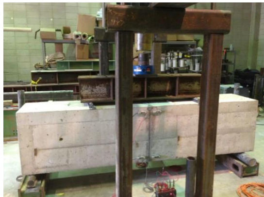
Figure 2.39 Specimen setup for static four-point bending test. (Hosteng, Phares, Abu-Hawash, Bierwagen, & Nelson, 2015)
