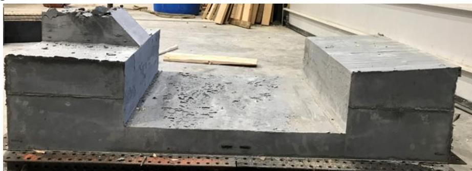
Figure 4.6 UHPC flowability test completed.
