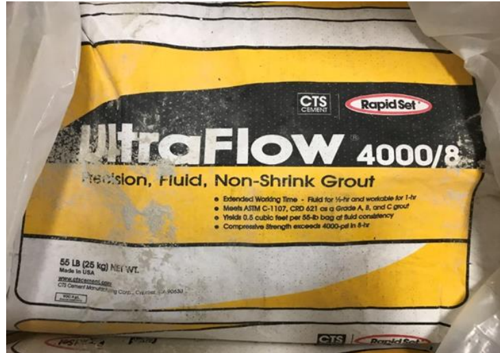
Figure 4.61 Non-shrink grout used for pile coupler grout bed.
