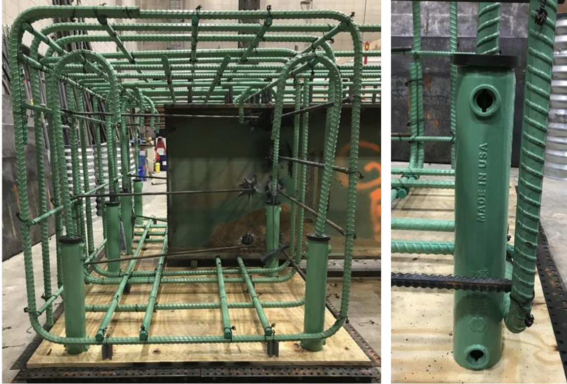
Figure 4.29 GRBC reinforcing cage with Dayton Superior grout sleeves.
