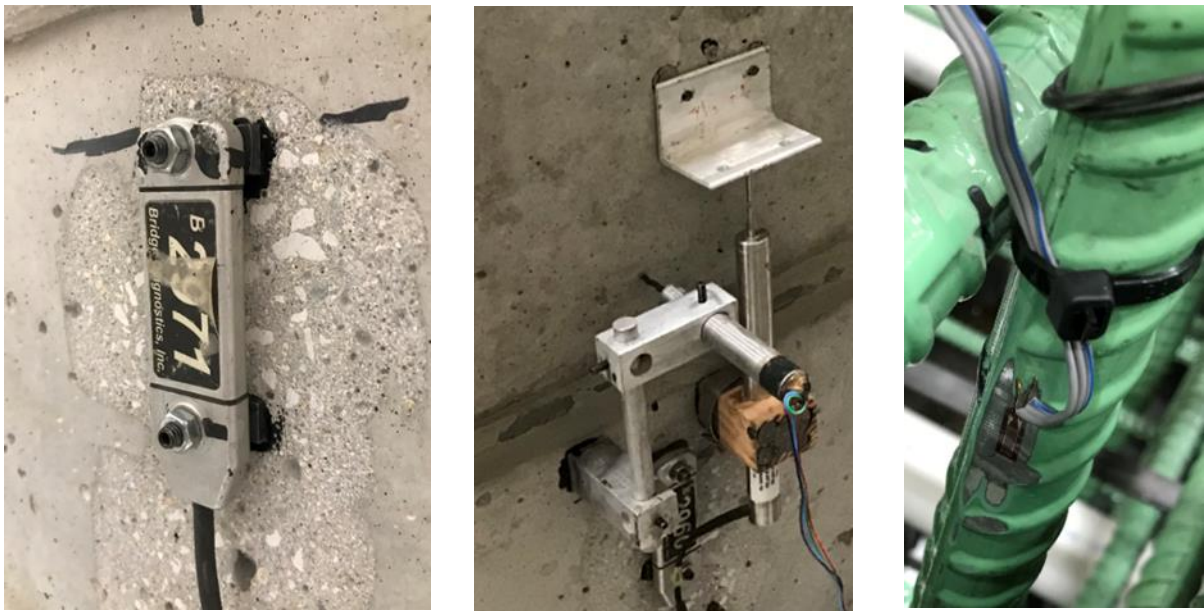
Figure 5.11 External strain gauge (left), vertical displacement transducer, horizontal displacement transducer, and external strain gauge (center), and sacrificial strain gauge (right).
