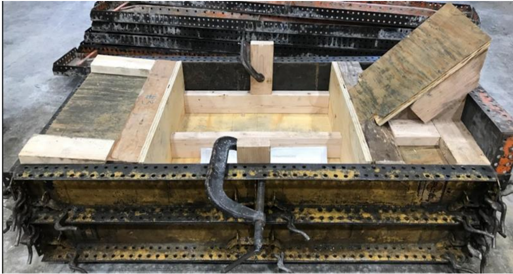
Figure 4.5 UHPC flowability test formwork.
