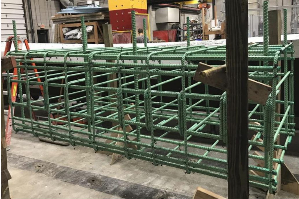
Figure 4.24 GRBC pile cap reinforcing cage.
