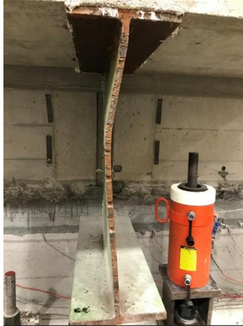
Figure 5.13 Beam buckling failure causing end of test.
