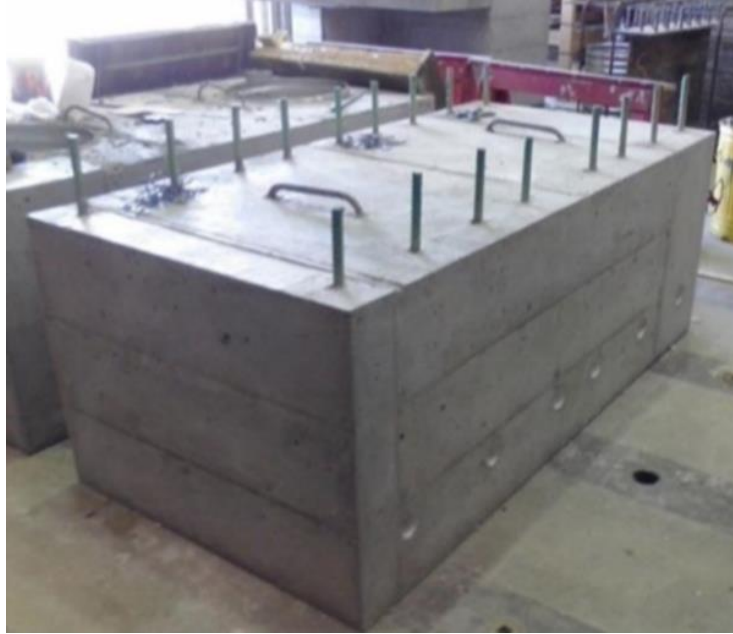
Figure 2.45 Grouted coupler pile cap. (Hosteng, Phares, & Redd, 2016)
