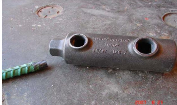
Figure 2.32 Lenton Interlok for #6 reinforcing bar. (Jansson, 2008)
